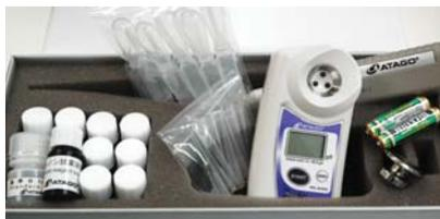
The kit comes complete with 10 bottles of quinone reagent solutions (5ml each), a micropipette, 10 micropipette tips, 10 disposable plastic pipettes, 1 bottle of calibration solution, an anti-volatile cover, and 2 AAA batteries.
