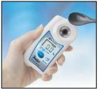
1) Place the sample onto the prism surface.
